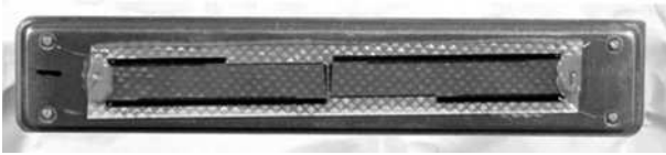
Figure 1.4 Surface-wave bandpass filter for a mobile phone basestation (courtesy of B. Abbott, Triquant).
