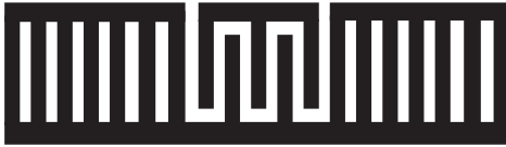
Figure 11.14 Synchronous resonator as impedance element.
